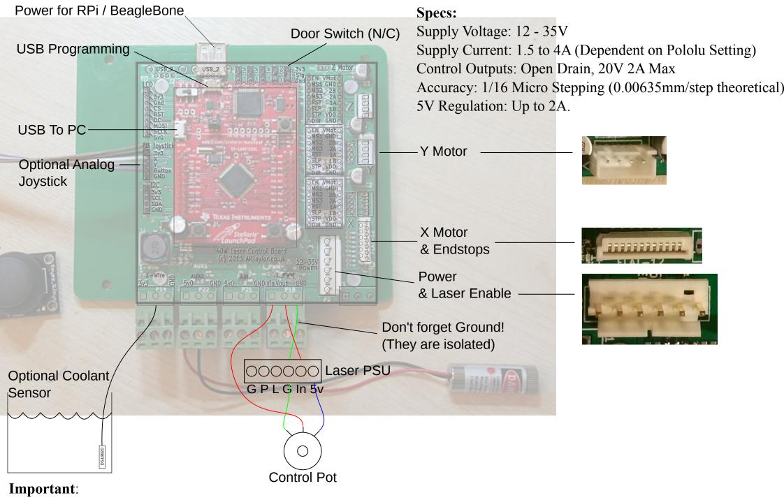
The default 24V PSU supplied with the laser is approaching its capacity. If powering other accessories from the same power source, please watch
